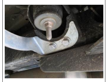
31.Using two M10 SEMS bolts and M10 flange nuts attach surround brace to chassis as shown. LHS shown finger tighten only.
