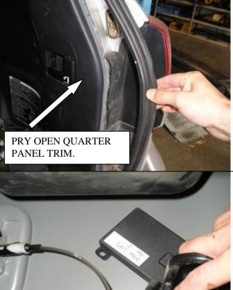
2. Carefully remove rubber trim surround being careful not to get any of the silicone on the vehicle interior. Once this is done remove the jack access panel and gently pry open the rear section quarter panel. Repeat for left hand side.
