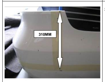
34. From edge of taillight section measure down 310mm and mark this point. Then using a length of masking tape join these points to form a straight line up to the recess for the fog light/ reflector.
