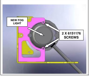
48. For vehicles equipped with factory fitted fog lights install kit 5715020.Remove centre piece of moulding by cutting with a 72mm hole saw using mould dimple on rear face as a centre point. Screw light to mount as shown and tap into original wiring loom by soldering extension provided in kit.
