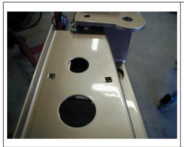
8. Fit M6 cage nuts (9 total) in square holes in top of bar as shown.
