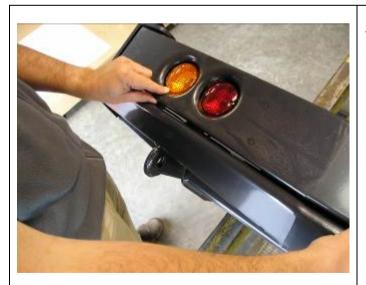
11. If a wheel carrier or jerry can carrier is not to be fitted a cover panel must be fitted.
