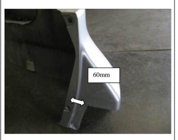
39. Tailgate side of bumper. Mark a line parallel to edge of rear face and inboard 60mm of bar up to previous marked line. Once all is marked cut using air hacksaw or similar and de-burr edges.
