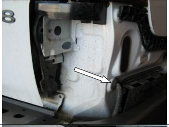
4. Locate factory rubber grommet on drivers side and remove. Pass section of loom with grommet attached through this hole making sure grommet seals tightly.
