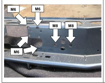
9. Fit M6 cage nuts (8 total) and M8 cage nuts (4 total) to front of bar. (RHS shown)
