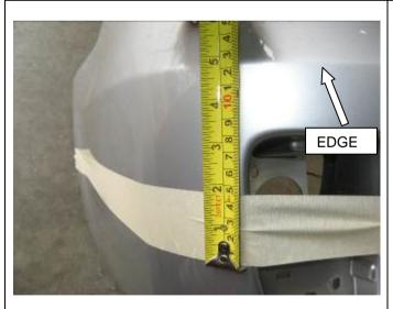
35. Measure 120mm down from mould edge in bumper to side of fog light/ reflector. Mark this point. Then using a length of masking tape join these points to form a straight line up to the recess for the fog light/ reflector. NOTE: Confirm line is straight by sighting down the length of bumper. If not readjust tape so a straight line is achieved.
