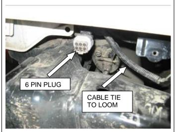
14. Locate and un-clip the 6 pin plug on the left hand side of the vehicle. Using cable ties supplied in kit attach it to loom that runs next to it making sure everything is clear of the exhaust.
