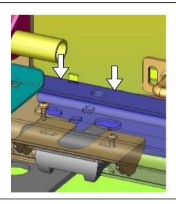
56. Fit trailer plug to recess using M5 pan head screws as shown by arrows.
