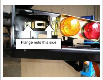
10. Fit locking pin brackets using two **M8 x 25 bolts**, flat washers and flange nuts. Finger tighten only.
