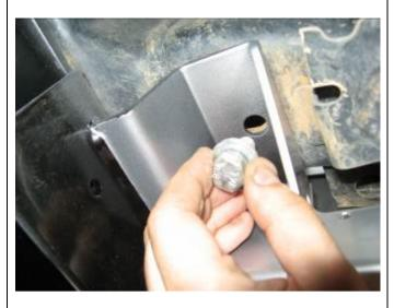
27. Secure bar to bottom of chassis and cage nut plates using 2 x M12 X 1.75 X 50 bolts, flat washers and spring washers. **Tighten all bolts when done**.
