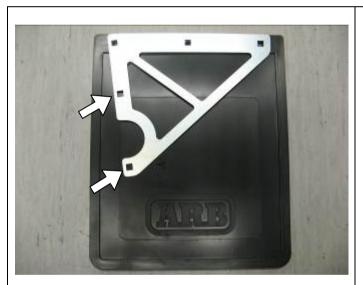
49. Place mounts on mudflaps as shown. On the ARB mudflap align the top holes of the mount with the top holes of the flap. Mark the two holes as shown in the photo and drill to 7mm. Install M6 cage nuts to holes in mount, LHS shown.
