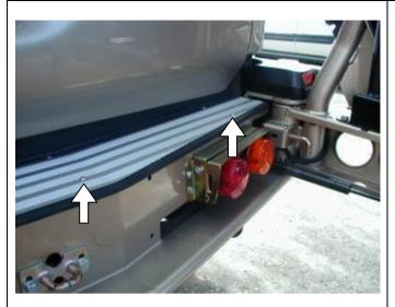
55.Using **M6 button head cap screws** fit aluminium step plate.
