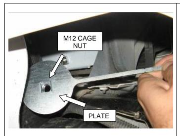
24. Fit M12 cage nut onto cage nut plates and insert through hole in side of chassis. Place one facing up and one facing down on each side. These are used to secure top and bottom inner mounts. **MUST BE INSTALLED BEFORE BAR IS MOUNTED.**
