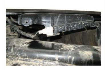
16. Locate steel bracket with plug attached on the left hand side of the vehicle. Un-bolt bracket from vehicle and retain hardware for next step.
