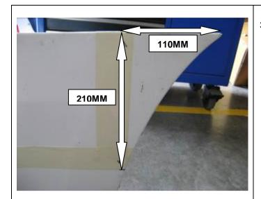
33.Remove fog light/ reflectors from rear bar. From top edge of wheel arch section measure back 110mm, then down 210mm. Mark this position.
