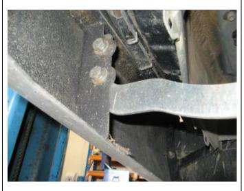
32. Using two M10 SEMS bolts and flange nuts attach surround brace to surround as shown. LHS shown finger tighten only.
