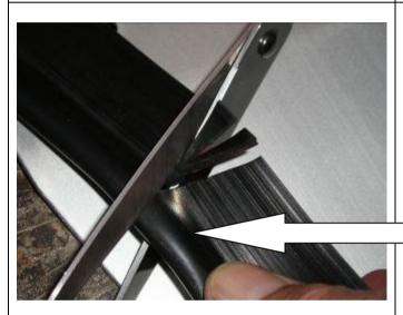
53. To fit rubber sealing strip to underside of aluminium step plate, lay strip on the underside of step plate and place so over hang is even on both ends. Using scissors, cut darts up to the bulb end of the rubber strip, so the strip can follow the front profile of the aluminium step plate.
