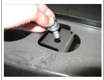
26. Secure bar to top of chassis and cage nut plates using 2 x M12 X 1.75 X 50 bolts, flat washers and spring washers.
