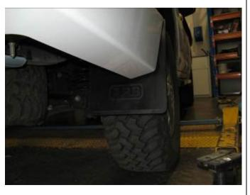
50. Place mudflap mount on inner surface of bar and mudflap on outer surface of bar and secure using black M6 bolts and flat washers.
