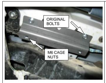
17. Attach two M6 cage nuts to new bracket supplied in kit. Fit bracket to vehicle using original bolts removed in step 16. Attach loom bracket to cage nuts using 2 x M6 x 16 bolts and flat washers.
