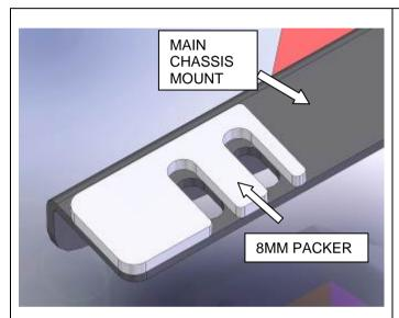
25. Place bar back on vehicle making sure there is enough clearance from step 23. When satisfied place the 8mm chassis packers on top surface of chassis mount and finger tighten only.
