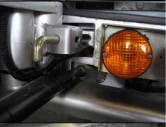
5. Run wires along rear of bar to corresponding lights. License plate light section is long enough to cover either fittment on drivers side or passenger side. Cable tie excess behind bar. Run tow bar wires down to plug in bar and secure.
