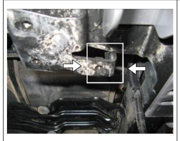
18. Locate right hand bumper bracket on underside of rear cross member. Area inside white box is to be trimmed to make way for rear bar mounts.
