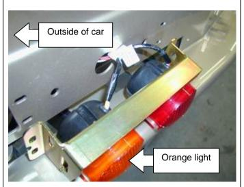
When fitting light assemblies to bar, orange (indicator) lights must be to the outside as shown. The flange on the bracket should also be at the top.
