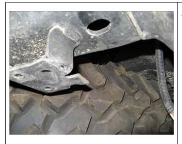
19. Trim bracket leg as shown using a small grinder with cutting disc or an air-hacksaw. Paint all bare metal surfaces after cutting.
