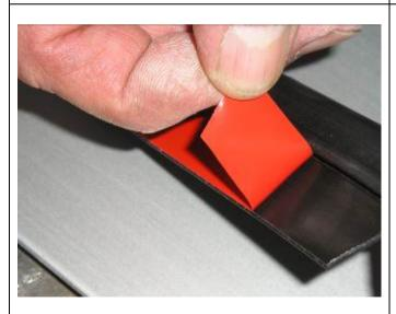
54. Carefully remove backing tape on the rubber strip and fit to step plate working from the centre outwards. Make sure rubber strip hugs the front edge of the aluminium step plate.
