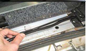
6. Run pick up wires for harness under bridging panel removed earlier to left hand side of vehicle. Secure with cable ties.
