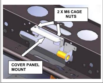
57. Install cover panel mount to cage nuts in bar using 4 x M6 x 15 bolts, spring washers and flat washers. Finger tighten only. Fit 2 M6 cage nuts to underside of mount. Close carriers if fitted and adjust mount to suit. Tighten all bolts.
