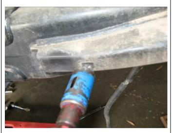
23. Drill the marked holes out using a 22mm hole saw. Clean up all burrs and paint.
