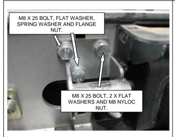
28. This bar is designed to make use of 100 SERIES carriers. Because of the different tow bar arrangement of the 200 SERIES new locating brackets have been supplied. If carriers are to be fitted install these now as shown for relevant sides. LHS shown. If carriers are not to be fitted keep these items for future use.
